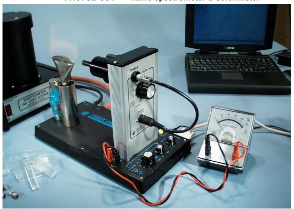
CH3792-001 flame spectrometer & colorimeter
